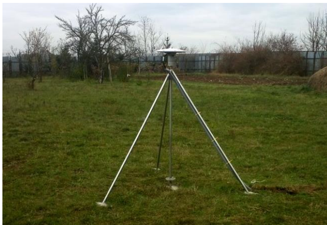
Obr. 1. Hĺbkovo vŕtaná stabilizácia bodu RISA Fig. 2. Deep drilled monumentation of the RISA station
