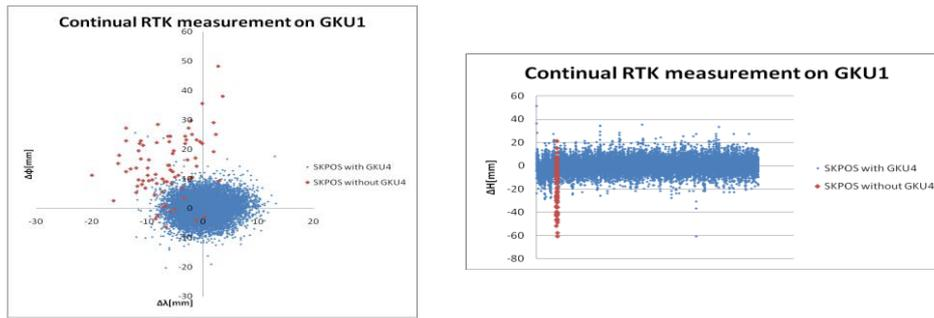
**Fig.3** Results from continual RTK measurement on GKU1 marker.
